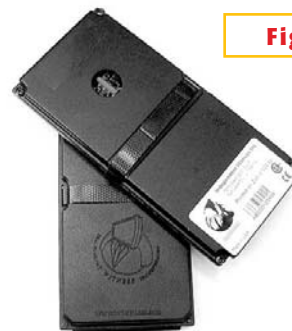
NASCAR uses the stand-alone Witness incident-data-recording system to build a database of crash information to improve driver safety.
