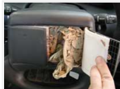
A rebuilder stuffed a used airbag back into the steering wheel on this retitled wreck.
