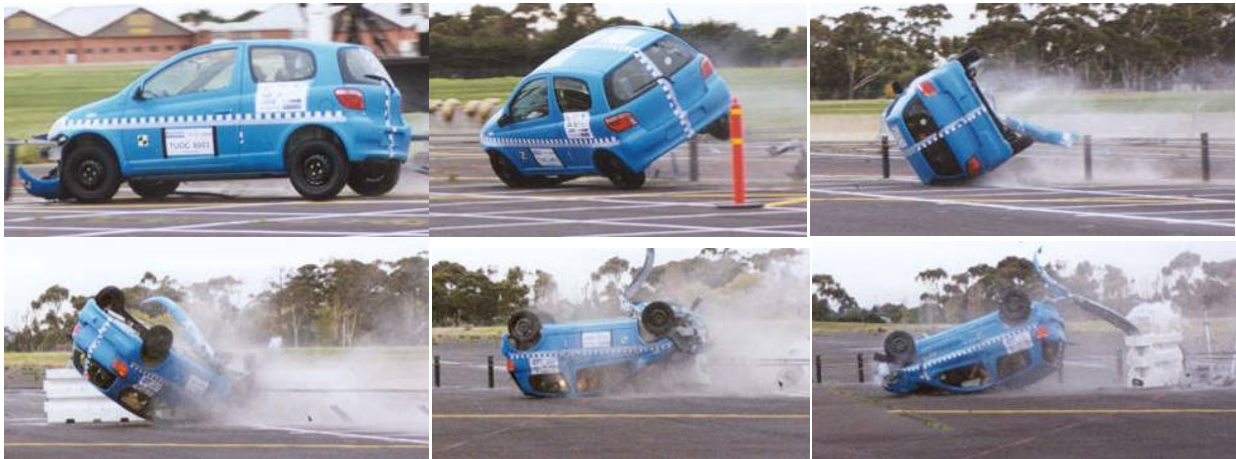
Figure 5 - Vehicle motion during typical longitudinal roll bounce-over initiated rollover (After Grzebieta et al) [20]
