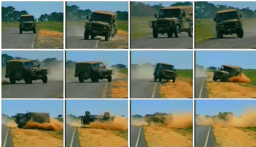
Figure 3 - Vehicle motion during typical trip initiated rollover (After Richardson et al) [19]
