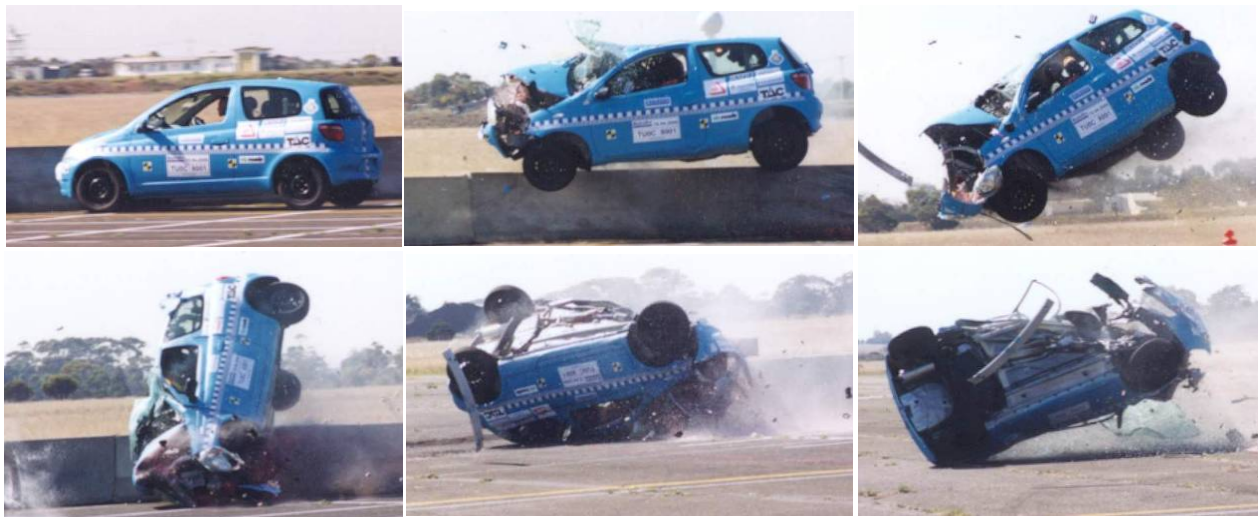
Figure 6 - Vehicle motion during typical End-over-end, bounce-over initiated rollover (After Grzebieta et al) [20]
