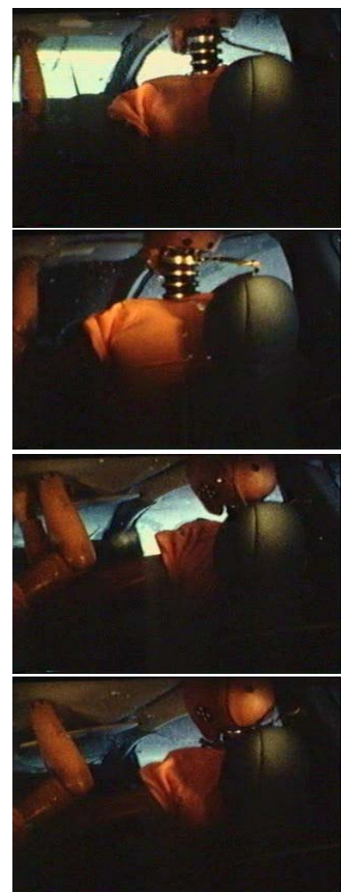
Figure 7– Screen captures of interior occupant motion of Toyota Echo rollover and high level of neck compression due to the roof deformation
