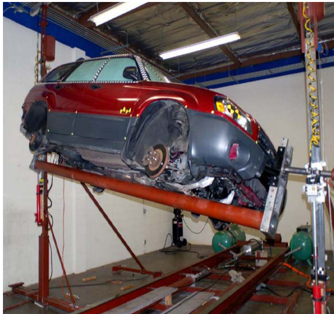
Figure 6: Photograph of the JRS Test Rig [Friedman et al, 2007b]
