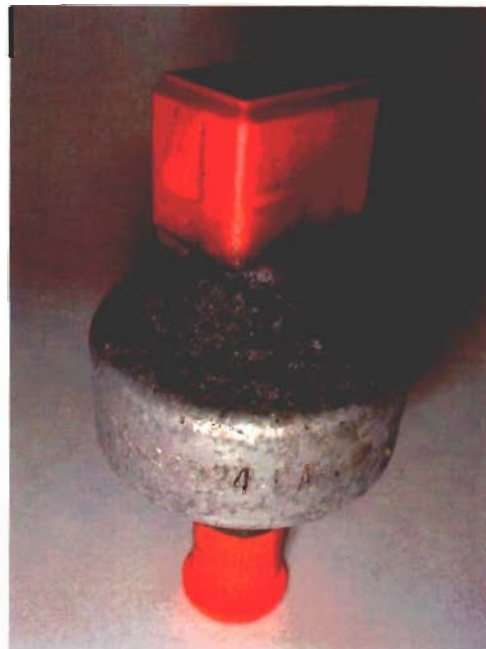
Figure 16. SCDS with melted base.
