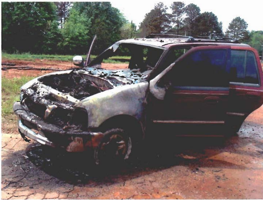
Figure 17. Burns Patterns On Test Vehicle.
