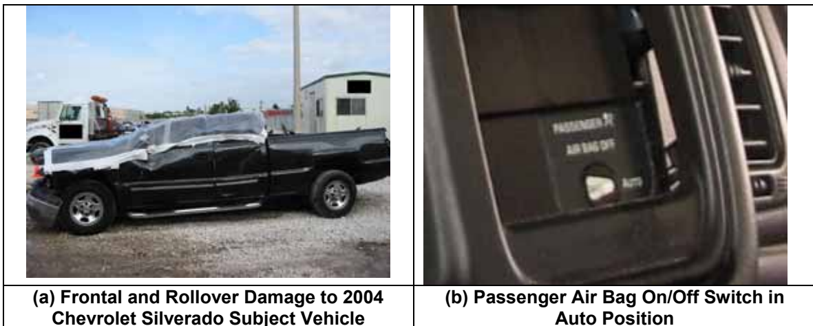
Figure 22. Frontal Crash Followed by a Rollover in Which Driver Air Bag Deployed, But Passenger Air Bag Did Not Deploy for a Child in the Right-Front Seat (NASS 2005-42-106)
